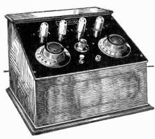
Type—Tuned Radio Frequency; Tubes—4; Battery—"A" Storage; "B" 90 Volts; Controls—Tuning, 2; Tube, 1; Dim.—14 x 14 x 10; Wt.—20 lbs.; Price—\$65.00.
