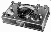
Electrical Instrument Works. By its use all the elements of a tube are tested—filament, grid and plate circuits. Curves can be plotted by the use of a C battery. Voltages of individual cells of A or B batteries can be measured or entire battery voltages measured in blocks of 22½ volts.
