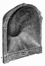
Trade Name—"Town Crier"; Material of Horn—Cement and other ingredients; Finish—Mahogany Crystal; Type of Magnet—Single Bar Tungsten; Action—Direct; Height—12¾ in.; Diameter of Bell, 9 in.; Weight—7½ lbs.; Price—\$17.50.
