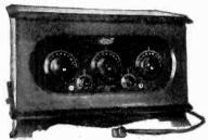
Trade Name — "No-Bat-Try"; Type — Tuned Radio Frequency; Tubes—5; Controls—Tuning, 3; Tube, 2; Dim.—24 x 14 x 1819; Wt.—40 lbs.; (operates directly from electric light socket entirely without batteries or battery eliminators); Price—A.C., \$130.00; D.C., \$180.00.
