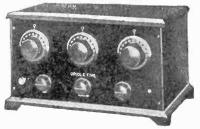
Trace Name - "Oriole Five"; Type - Tuned Radio Frequency; Tubes—5; Battery—"A" Storage or Dry; "B" 90 Volts; Controls—Tuning, 3; Tube, 2; Dim.—15 x 17 x 9; Wt.—20 lbs.; List Price-\$47.50.
