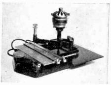
with any 110-volt outlet. Operation is upon the pantagraph principle, a guiding stylus being mounted upon an extension arm which is moved by the operator, either through master letter dies furnished with the machine or over a design previously marked out. This machine is being distributed by the Service Radio Corporation, 119 West Nineteenth Street, New York.
