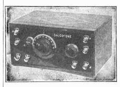
Trade Name — "Dalcofone"; Type — Radio Frequency; Battery—"A" Storage or Dry; "B" 90 Volts; Tube—1; Controls—Tuning, 1; Tube, 1; Antenna—Outdoor; Dim.—11½ x 5½ x 7; Wt.—3 lbs.; Price—\$8.75.
