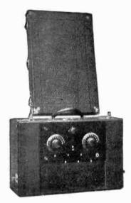
Trade Name—"Concert Sr."; Type—Reflex; Tubes—2; Battery—"A" Dry; "B" 90 Volts; Controls—Tuning, 2; Tube, 1; Antenna—Indoor or Loop; Dim.—13 x 11 x 19; Wt.—25 lbs.; Price—\$75.00.
