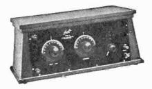
Trade Name -- "Wright"; Type -- Radio Fre uency; Tubes-2; Battery-"A" Storage or Dry "B" 45 Volts; Controls-Tuning, 2; Tube, 1 Antenna-Outdoor; Dim.-5 x 16; Wt.-10 lbe. Price-\$50.00.
